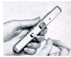
Clean lens window with cotton swab - or with a clean linen cloth wrapped around a match or wood stick.
